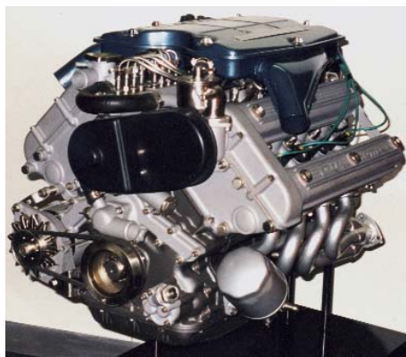
Mechanical fuel injection, tungsten crankshaft counterweights and a dry sump make for a compact motor
