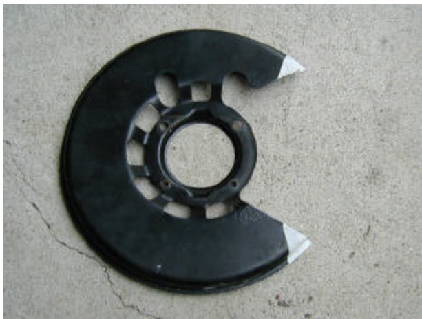
Picture 5 Dust shield marked for trimming
