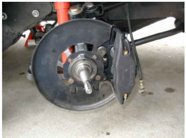
Picture 4 dust shield and caliper installed
