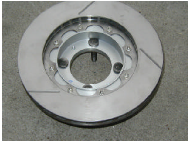
Picture 2 Custom rotor and hat, rear
