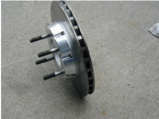
Picture 3 Custom rotor and hat, side
